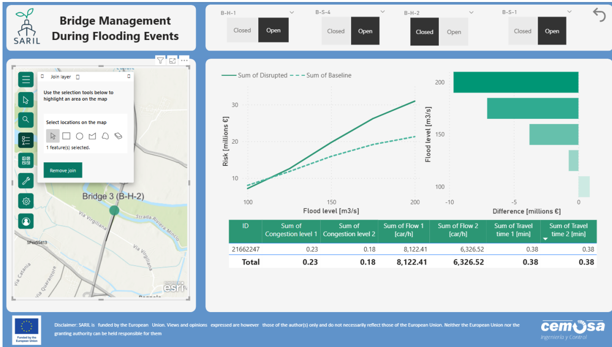
Figure 13: Bridge management during flooding events. Interconnection between data simulation outputs and geographical context.
